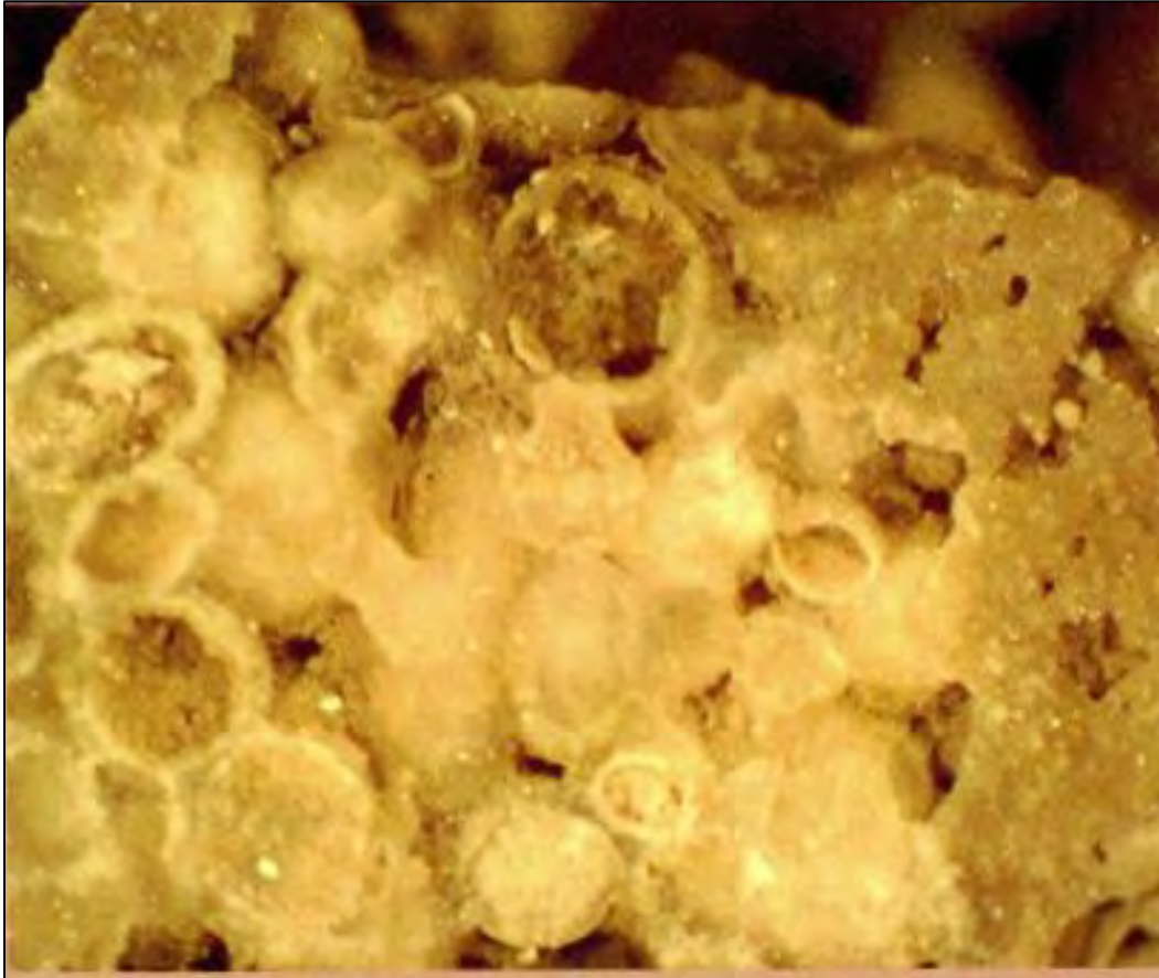
Intergranular oolitic and moldic porosity
